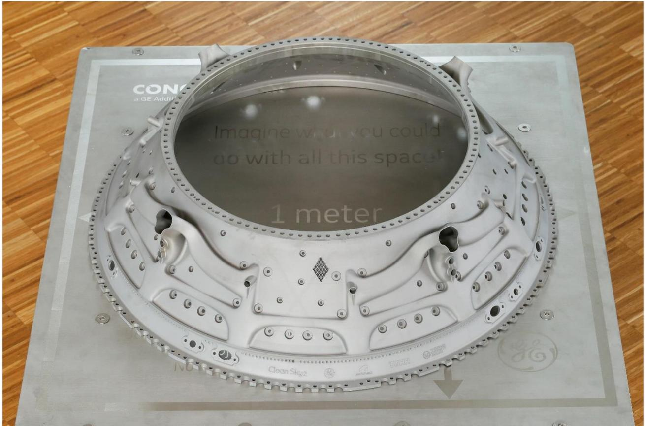
Equivalent to one meter in diameter, the first-ever metal 3D-printed TCF casing using DMLM technology in nickel alloy 718. Image credit: GE Aerospace. (Photo: GE Additive, GEADPR067)
