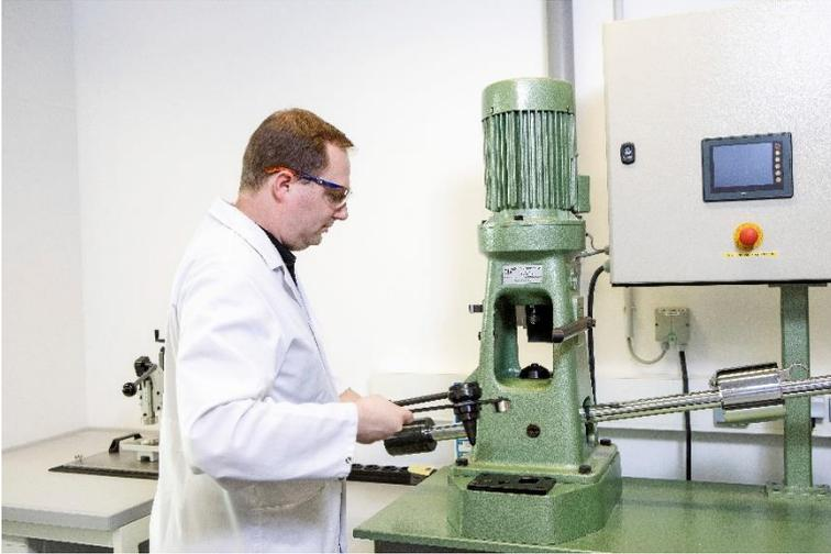
Welding load measurement of phosphorous additives in fully synthetic formulations.
