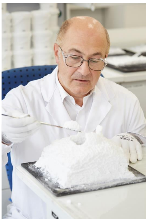
Exolit® AP flame retardant grades based on ammonium polyphosphate have become the industry standard in intumescent coatings formulations. Steel plate protected with intumescent coating after a fire test. (Photo: Clariant)
